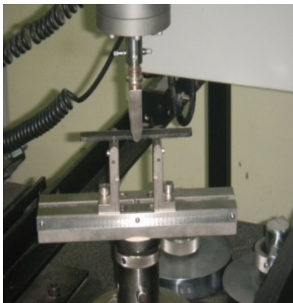
Fig. 2 (a). Flexural Testing
