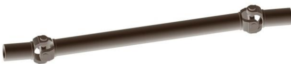
Fig.5 Assembled Propeller Shaft with U-Joint
