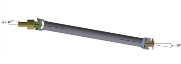
Fig.10 Propeller Shaft System at Operating angle \alpha = 10^\circ
