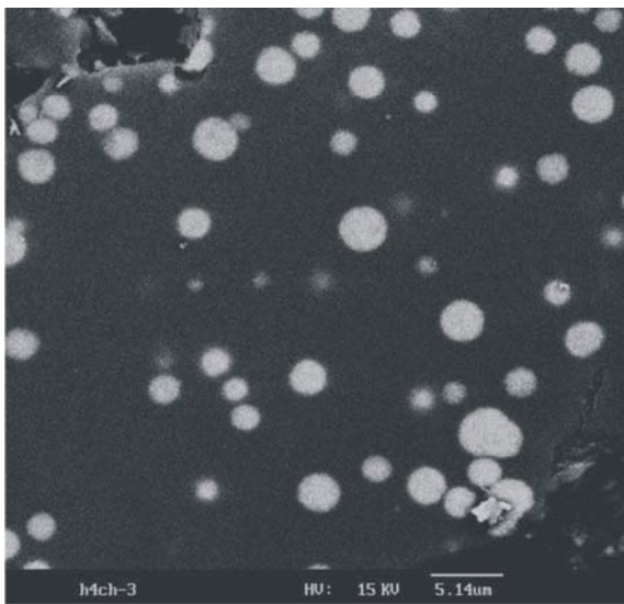
Fig.1. SEM morphology of cordierite and CeO 2 Sample
