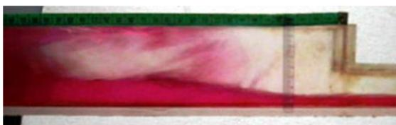
Fig.15. Slug flow in suddenly expanding channel
