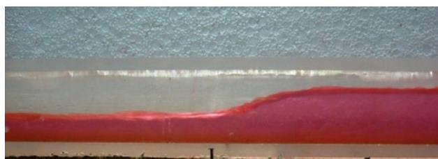
Fig.7. Hydraulic jump in a horizontal test-section without air flow ( $Q_w=2.0 \times 10^{-4} \text{ m}^3/\text{s}$ ,  $Q_a=0.0$ ), ( $h_1=10 \text{ mm}$ ,  $h_2=30 \text{ mm}$ )
