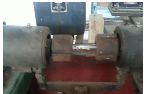
Figure 9: Process Setup for Fatigue Test, Civil Engineering Lab, Pravara Rural Engineering College, Loni.
